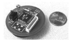
Fig. 8. A TinyOS-based mote. This "mote" includes a 4 MHz microcontroller, a software-driven radio, and an application that coordinates with neighboring motes to discover an ad hoc sensor network routing topology.
