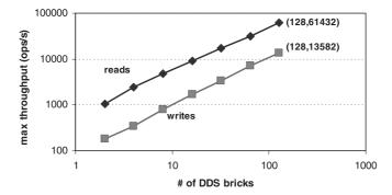
Fig. 6. Throughput scalability. This benchmark shows the linear scaling of throughput as a function of the number of bricks serving in a distributed hash table; note that both axis have logarithmic scales. As we added more bricks to the DDS, we increased the number of workers using the DDS until throughput saturated.
