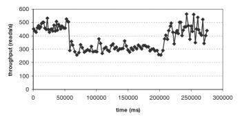
Fig. 7. Availability and recovery. This benchmark shows the read throughput of a three-node hash table as a deliberate single-node fault is induced, and afterwards as recovery is performed.
