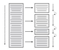
Fig. 2. Splitting a service into stages. Our programming model views a service as a sequence of stages, separated by high- or variable-latency operations. Stages only share data using pass-by-value semantics, for example, by exchanging messages.
