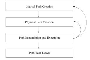
Fig. 11. *Path construction process*. Path execution is an iterative process of optimization. The Ninja APC facility guarantees the availability and fault-tolerance of a constructed path by rebuilding its physical or logical path.
