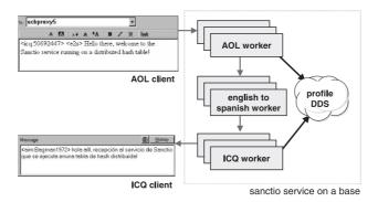
Fig. 15. Sanctio messaging proxy. The Sanctio messaging proxy service is composed of language translation and instant message protocol translation workers in a base. Sanctio allows unmodified instant messaging clients that speak different protocols to communicate with each other; Sanctio can also perform natural language translation on the text of the messages.
