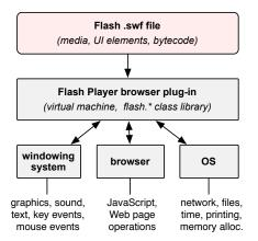
Figure 1: Flash architecture. A Flash program is contained within a .swf file, and is executed by a virtual machine implemented by the Flash Player browser plug-in. The Flash Player also defines a set of classes that allow the Flash program to interact with the host OS, its windowing system, and the Web page and browser in which the Flash program runs.
