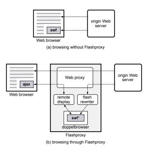
Figure 2: High-level Flashproxy architecture. (a) A browser directly fetching a Web page with an embedded Flash program. (b) A browser using Flashproxy to fetch the same Web page; Flashproxy rewrites the Web page, replacing the Flash program with a remote display AJAX component. The Flash program executes within a "doppelbrowser" – a full Web browser and Flash Player executing in Flashproxy.
