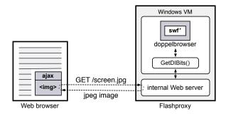
Figure 5: Remote display. Flashproxy uses the GetDIBits Windows system call to grab screenshots of the Flash program executing in the doppelbrowser on a Windows VM. The remote display AJAX component on the user's browser pulls screenshot updates from the Flashproxy internal Web server.
