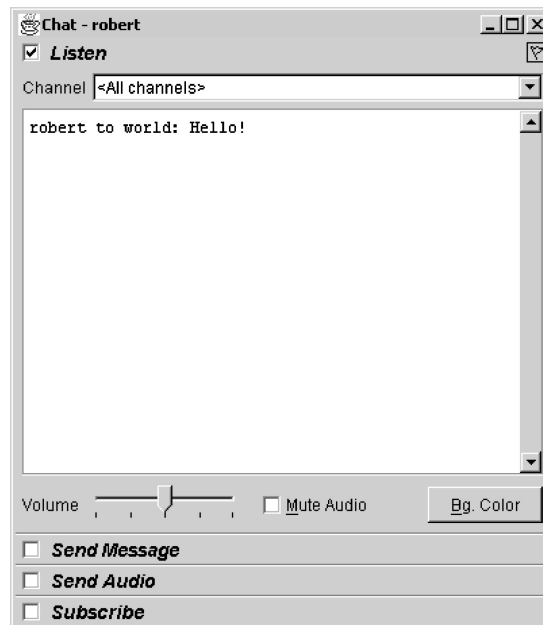
Fig. 18. A screenshot of Chat’s user interface. The user interface is divided into four panels, which can be independently expanded or collapsed by checking or unchecking the corresponding checkbox. The listen panel shows received text messages and provides volume control for audio playback. The send message panel lets the user send text messages, and the send audio panel lets the user send audio, either from a microphone or from stored audio tuples. Finally, the subscribe panel lets the user select the channels she is currently listening to.
